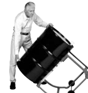
Push drum back on stand and grasp top and bottom chime
